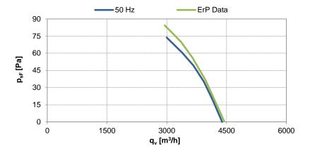
Fan characteristic measured in short bell mouth with guard grill ErP characteristic measured in full bell mouth without guard grill
