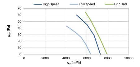
Fan characteristic measured in short bell mouth with guard grill ErP characteristic measured in full bell mouth without guard grill
