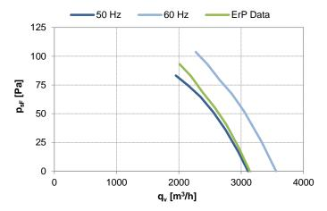
Fan characteristic measured in short bell mouth with guard grill ErP characteristic measured in full bell mouth without guard grill
